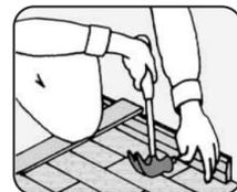
12. When the glue hardens (two-three hours), the wedges shall be removed and dilation gaps shall be covered with friezes and ledges.
