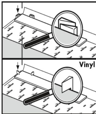
✓ Put spacers between the planks and the wall when installing your floor. They provide a uniform and sufficient expansion joint of 8 to 10 mm/0.32 to 0.39in.. Place the spacers about every 30 cm/ 1 ft.
