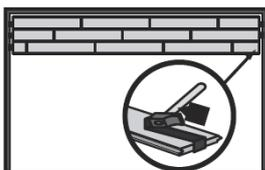
✓ Sometimes the tapping block cannot be used if there is not enough space (e.g. against the wall or under a radiator). The Quick-Step® crowbar is ideal for these situations. To place the plank correctly, put the Quick-Step® crowbar over the edge of the plank and tap the plank into the correct position with a hammer.
