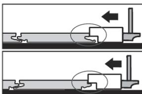
✓ Place the Uniclic tapping block with the groove on top of the plank tongue and tap the planks into the correct position with a hammer.
