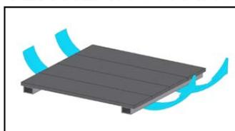
It is essential to ALWAYS leave an airspace between the staves and the supporting surface to allow ventilation. In addition to the use of a proper subconstruction framework it is necessary to avoid interferences between the airspace and edges or barriers that block a proper ventilation under the profiles. In case of hollow profiles it is recommended to make sure that there is no stagnant water inside the hollows.
