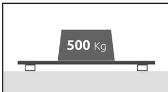
Floors constructed with Novowood staves, both filled and hollow core, combined with joists and fixed with Novowood Clips, laid with joists with a spacing of 35cm (~1ft 2in), are designed to support accidental overloads with resistance to distributed loads equal to 500 kg/m<sup>2</sup> (~102 lb / sq ft). In case of big loads on the decking and in all the public spaces, it is necessary to lay the joists with a maximum spacing of 30 cm (~11 13/16 in).
